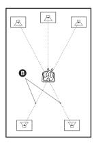
$[L/R] \frac{3.0 \text{ m/}10 \text{ ft}^2)^3$ : Set the surround speaker distance (up to 5.0 meters (16 ft) closer to the front speakers).
